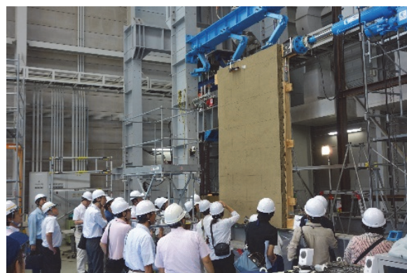
Production of mud walls and horizontal load testing
