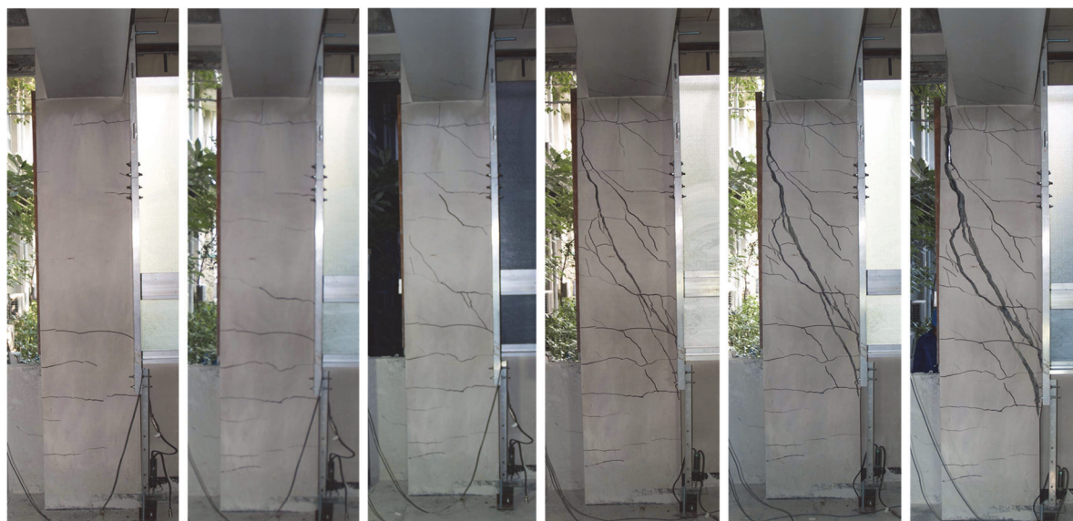
Figure 5.4.1 The progression of the inter-story drift angle ( R ) and the transition of the destructive behavior for a column in the 1st story of an existing 3-story reinforced concrete building under horizontal loading experiment: (From left to right: R = 0.2, 0.4, 0.67, 1.0, 1.5, 2.0 \times 10^{-2} radians.) 3)
