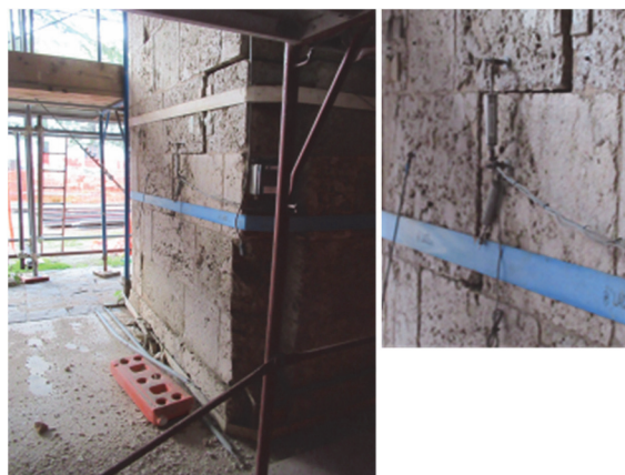
Figure 5.6.1 Crack displacement monitoring at the Spanish castle damaged by the L'Aquila Earthquake
