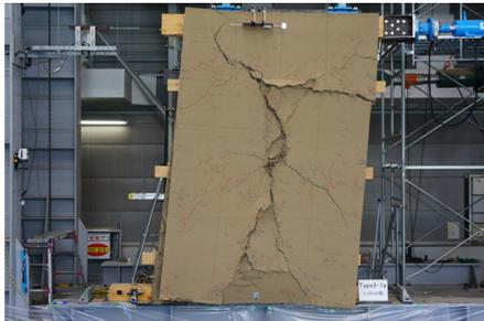
Figure 3.6 Testing structural strength of an earthen wall seen in storehouses
