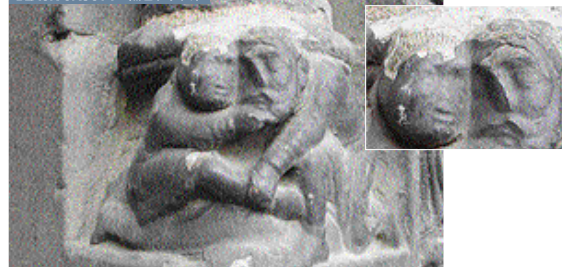
Black crust tracing the surface of a limestone sculpture.
